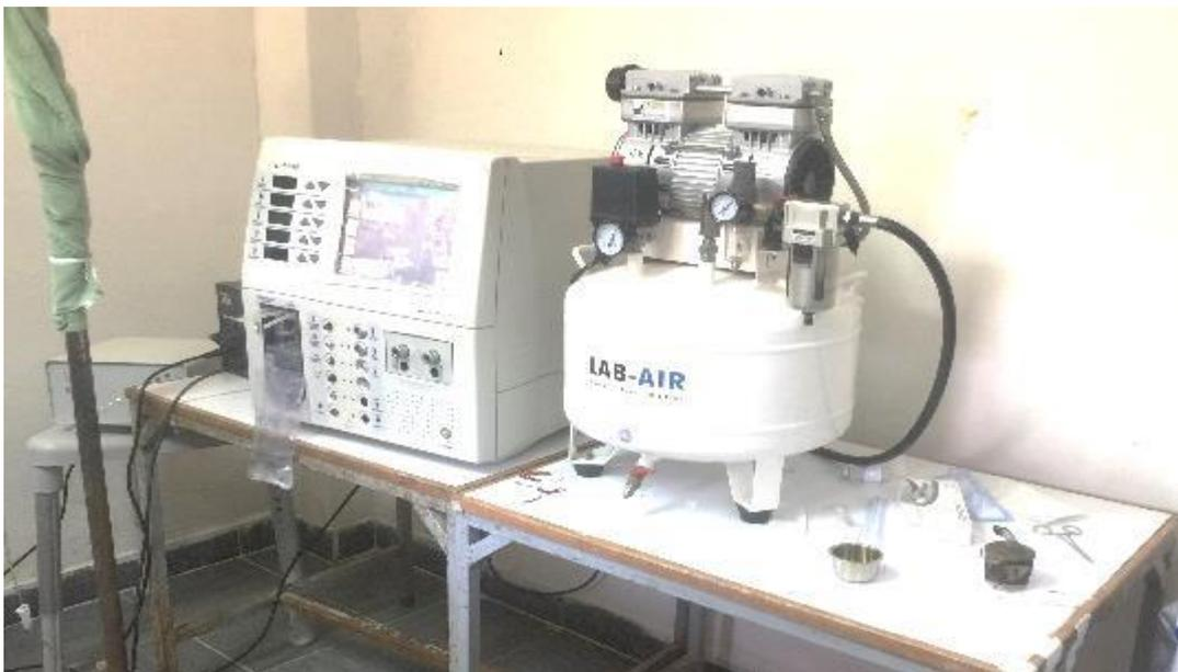
***Sophisticated vitrectomy machine we would not make work. Vitrectomy machine Compressor and air reservoir without which vitrectomy machine will not work. Much simpler Geuder vitrectomy machine which worked fine once we found the foot pedal***
