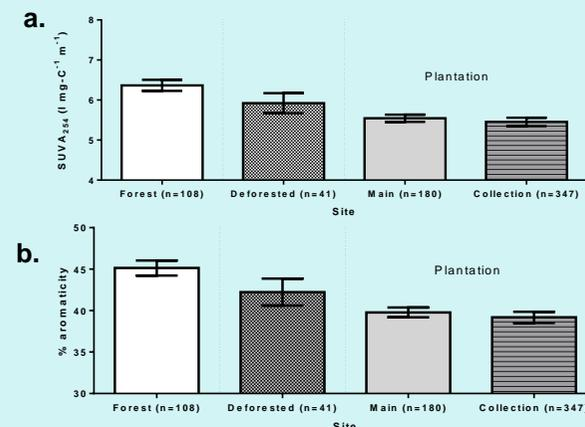
**Figure 4.** Mean (a) SUVA<sub>254</sub> data and (b) percent aromaticity data for the main and collection drains within the plantation estates and the forest sites from, August 2015 – April 2016. Bars indicate standard error of the mean. \* Percent aromaticity was calculated using the equation outlined in Weishaar et al (2003);  $Aromaticity (\%) = (6.52 * SUVA_{254}) + 3.63$
