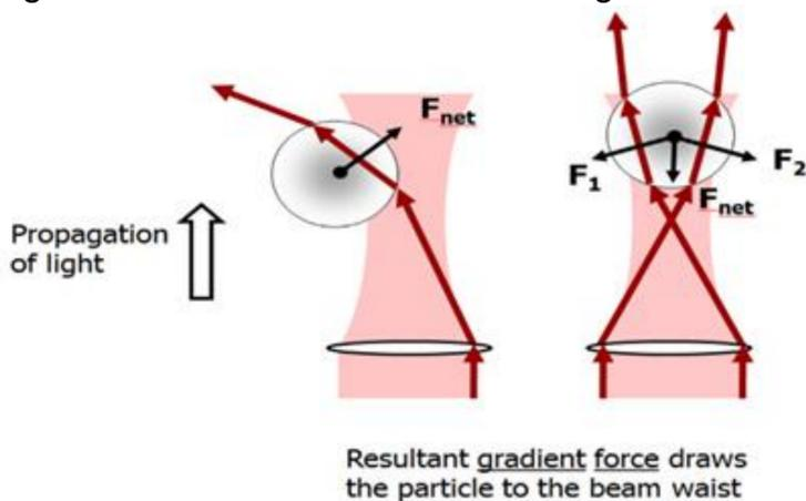
Figure 1 – An optical trap.
