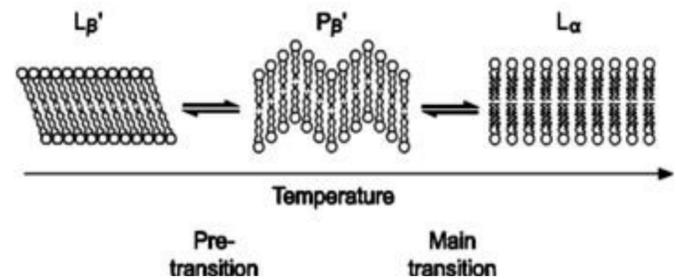
Figure 3 – A liposomes temperature transition. As the liposome transitions the tails switch from being compact and ordered to being loose. Image taken from [1].
