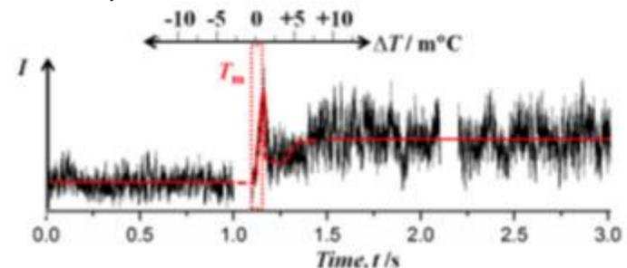
Figure 5– High resolution light scattering from the liposome against time.
