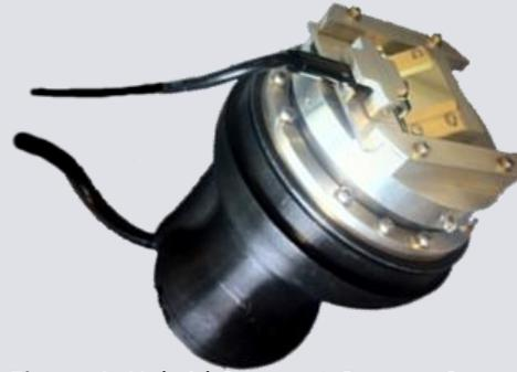
Figure 1: Hybrid Compact Gamma Camera (HCGC)
