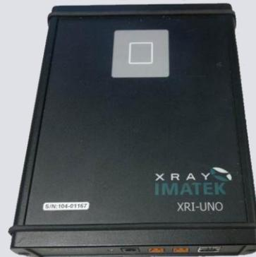
Figure 2: XRI-UNO CdTe detector
