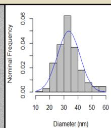
Figure 2: Size distribution of the nanoparticles as measured from TEM images (left). The mean diameter for these samples is 34 nm.
