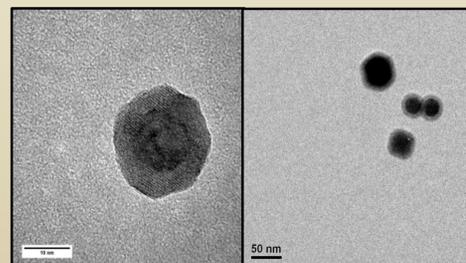
Figure 1: TEM images of suspected aluminium coated Fe nanoparticles produced using the gas-phase synthesis method explained above. It has been shown that the heating anneals the nanoparticles and changes their shapes and properties. [2]
