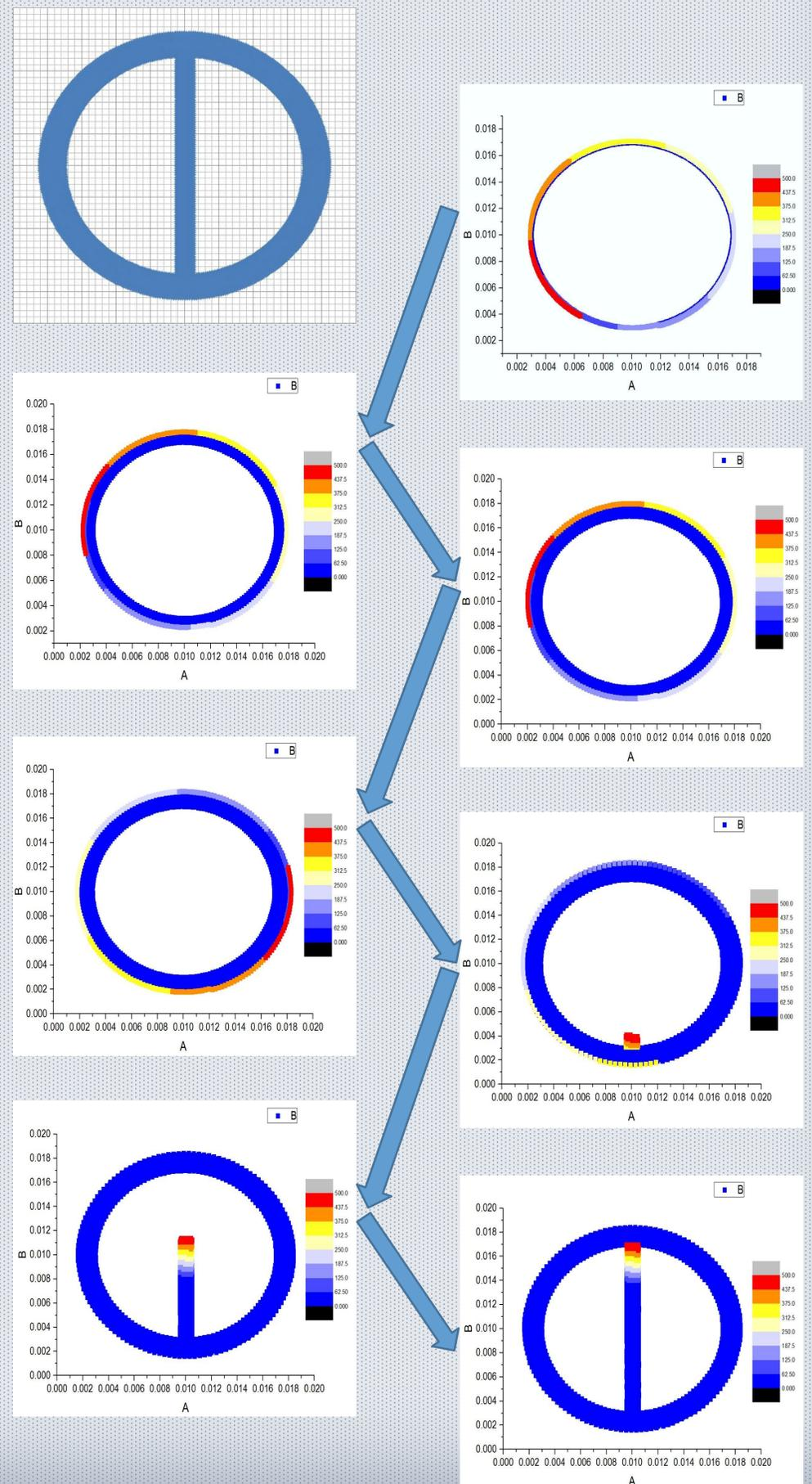
Stress analysis with respect to time and laser spot movement in 2D.
