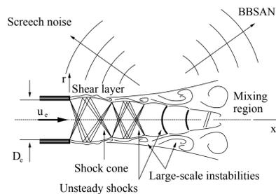
**Fig. 1: Under-expanded jet**
