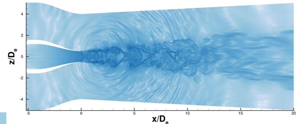
**Fig. 3: Pseudo-schlieren visualisation of a 3D jet simulation**
