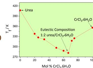
**Fig 9:** The phase diagram of the system
