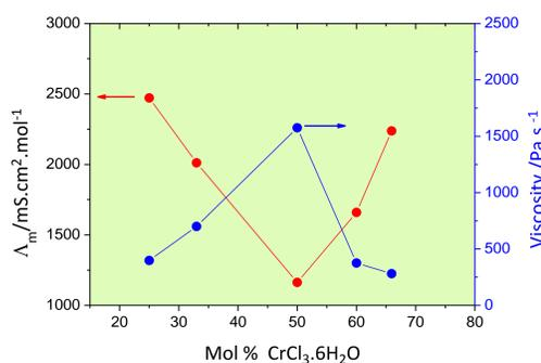
**Fig 6:** Molar conductivity vs. viscosity of urea /  $\text{CrCl}_3 \cdot 6\text{H}_2\text{O}$  as a function of temperature and compositions
