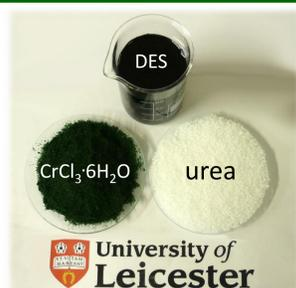
**Fig 1:** The new DES and its two solid components.
