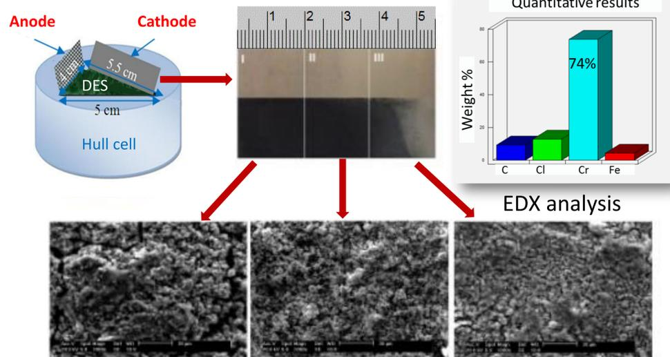
**Fig 10:** Bulk deposition from the 1:2 urea /  $\text{CrCl}_3 \cdot 6\text{H}_2\text{O}$  system at 40 °C for 1 hour onto a mild steel electrode at a current density of 0.2 mA/cm<sup>2</sup> resulted in an amorphous black deposit of ~65 μm thicknesses.
