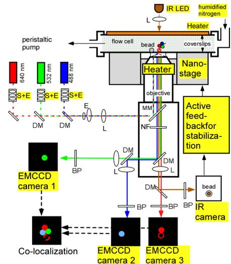
**Fig. 3.** Three-colour TIR fluorescence imaging instrument. Abbreviations: IR LED, infrared LED; MM, multichroic mirror; NF, notch filter; DM, dichroic mirror; BP, bandpass filter; S, beam shaper; E, beam expander; L, lens. Modules for stabilization and multiplexing are in yellow. Stabilization is achieved by IR bead tracking.
