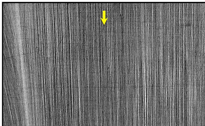
**Fig. 1.** Suction Surface Flow Visualization between 80% and 95% Axial Chord of NRC Turbine Blade at a Discharge Mach Number of 1.16.
