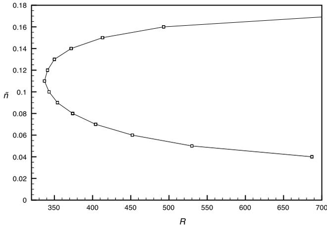
Fig. 3. Neutral curve for the onset of linear global instability.
