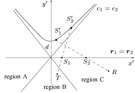
Fig. 3. The diffraction points  $S_1$  and  $S_2$  are obtained imposing the alignment of  $T, S_1, S_2$  and  $R, S_2, S_1'$ . For future reference, the half-plane  $y' < 0$  is subdivided into three regions determined by the asymptotes of the hyperbole.
