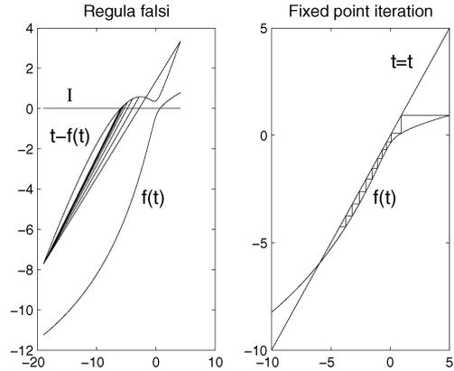
Fig. 6. Few iterates of both the regula falsi (left) and fixed point (right) algorithms given the same data configuration.
