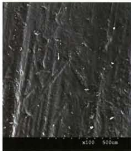
FIG 2c – SEM image of microwear on a cast made from a Speedex Light mould
