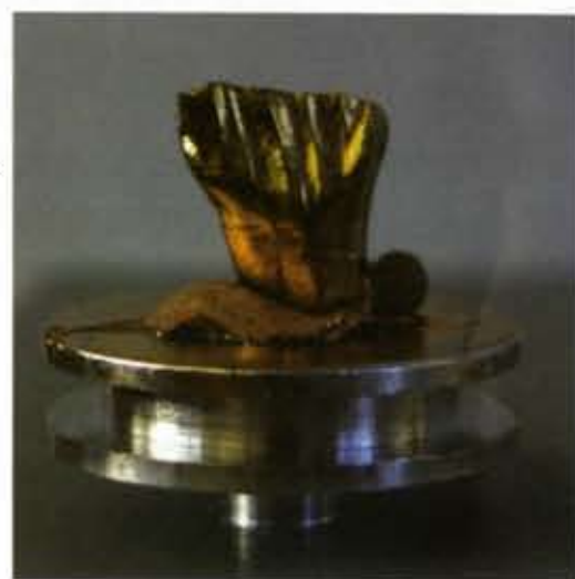
FIG 1c – Araldite 20/20 cast of Hypsilophodon foxii tooth, made from Speedex Light mould, mounted on SEM stub and splutter-coated with gold
