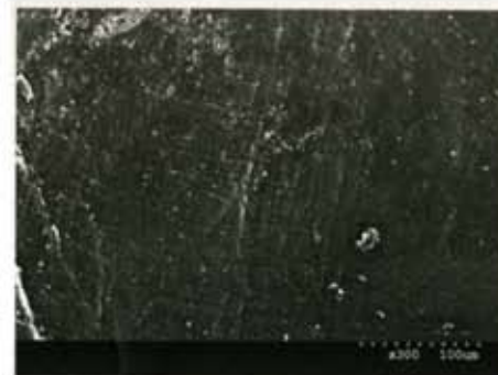
FIG 3c – SEM image of microwear on a cast made from a Speedex Light mould
