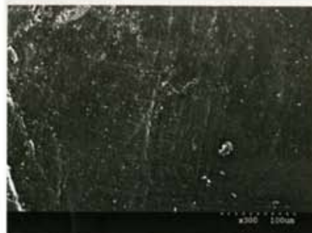
FIG 3b – SEM image of microwear on a cast made from a Speedex Light mould
