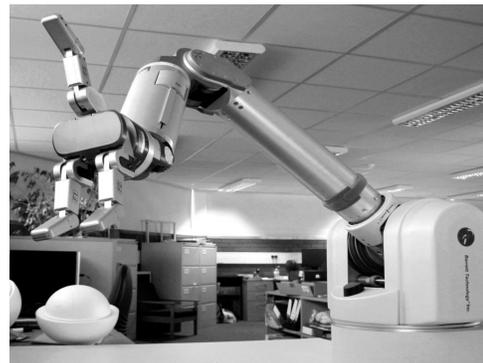
Fig. 1. The Barret 7-DOF Whole Arm Manipulator with the BH8-series BarrettHand.
