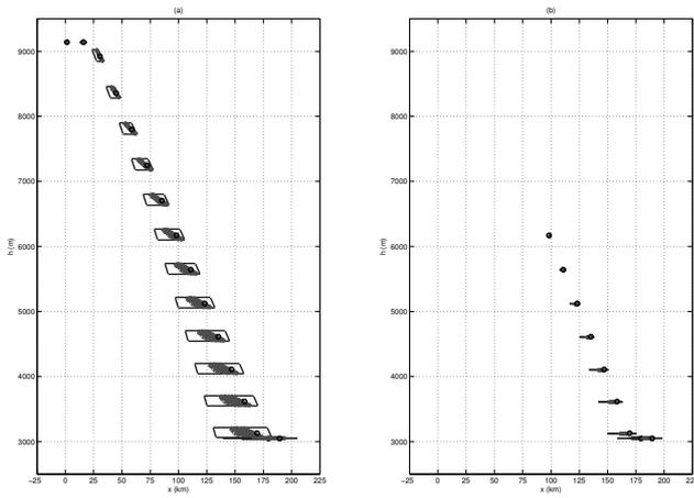
Fig. 5. Trajectory predictions drawn every 60 sec: (a) initial predictions; (b) half way predictions. The circles represent the real position, the grey dots represent the most probable positions, and the lines represent the worst-case prediction sets.
