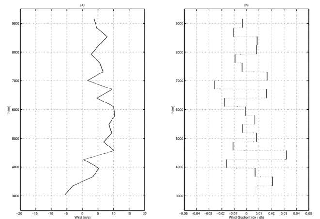
Fig. 2. (a) a possible realization of the wind profile; (b) the corresponding realization of the gradient of the wind with respect to altitude.
