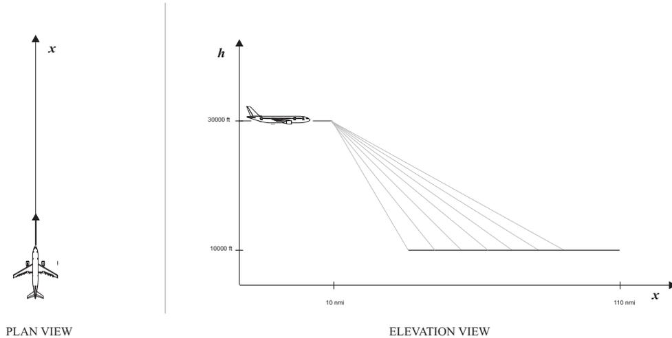
Fig. 1. The leg of flight of interest in the  $x$  (forward displacement) and  $h$  (altitude) coordinate system adopted in the case study. Uncertainty in the prediction of the displacement of the aircraft along the  $x$ -axis is due to the action of the winds, inexact knowledge of the mass of the aircraft and observation errors.
