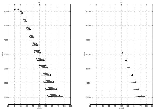
Fig. 6. Trajectory predictions in the actual worst case drawn every 60 sec: (a) initial predictions; (b) half way predictions. The circles represent the real position, the grey dots represent the most probable positions, and the lines represent the worst-case prediction sets.
