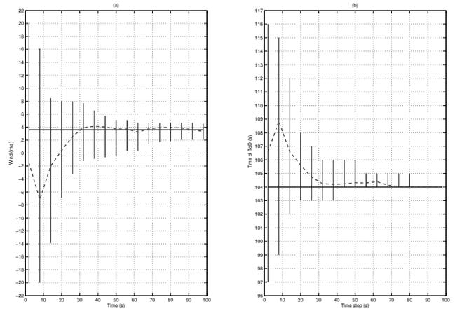
Fig. 4. (a) estimate of the wind speed during the initial phase in level flight; (b) prediction of the instant of the Top of Descent (ToD). In both figures: the bold line represents the actual value, the dashed line represents the expected value, and the vertical lines represent the worst-case estimate, or prediction, intervals.
