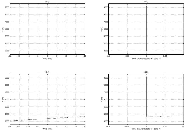
Fig. 3. (a1-a2) worst-case wind profile that gives the maximum forward displacement; (b1-b2) worst-case wind profile that gives the maximum airspeed at the end of the prediction horizon.
