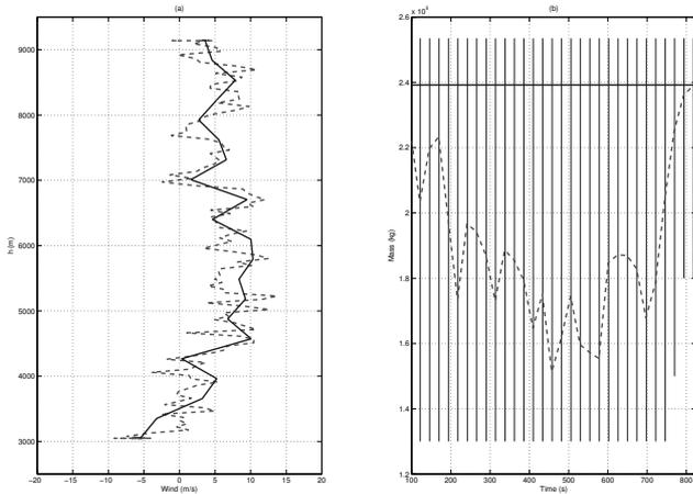
Fig. 8. (a) estimation of the wind profile: the bold line represents the real wind profile, the dashed line represents the expected value; (b) estimation of the mass during the descent: the bold line represents the real value of the mass, the dashed line represents the expected value, and the vertical lines represent the worst-case uncertainty intervals.
