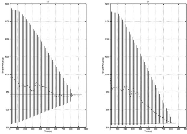
Fig. 7. Evolution of the predicted time of arrival during the flight: (a) in the case illustrated in Figure 5; (b) in the case illustrated in Figure 6. The bold line represents the actual time of arrival, the dashed line represents the expected time of arrival, and the vertical lines represent the worst-case prediction intervals.
