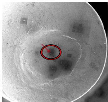
Optical zoom onto the pin head (150x)
